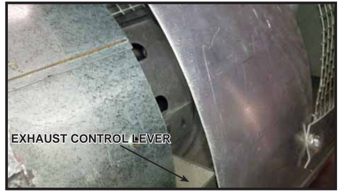
Figure 7.10 PVK-80 Control Lever Adjustment - Open
